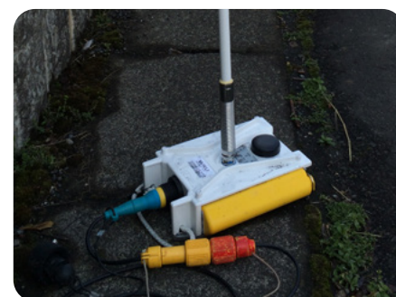
Wireless Remote Units (WRUs) being deployed in the field.
